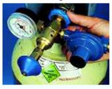
4 Slowly open the cylinder valve by turning it in an anti-clockwise direction. When gas is flowing through to the filling kit a click can be heard.
